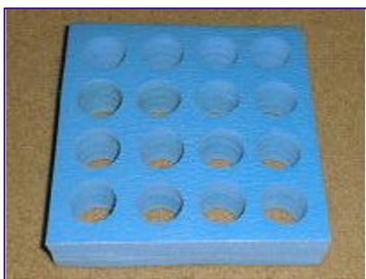
Similar results might be obtained with a hole saw (*without* the center drill bit) running at very high speed. I did not try that method. *Do not attempt drilling foam with a twist or spade drill.* It will just wrap the foam onto the drill bit and could cause injury if your are holding the work by hand.
