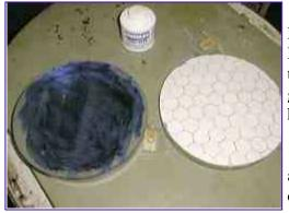
In use, I simply paint the whole surface of the optic with Dykem, let it dry thoroughly, and then grind for a couple of wets. During the first wet, you can easily observe the wear patterns of the tool on the optic just as you would when watching a Sharpie grid marked on the component. The Dykem easily shows exactly how good contact is during the wet.
